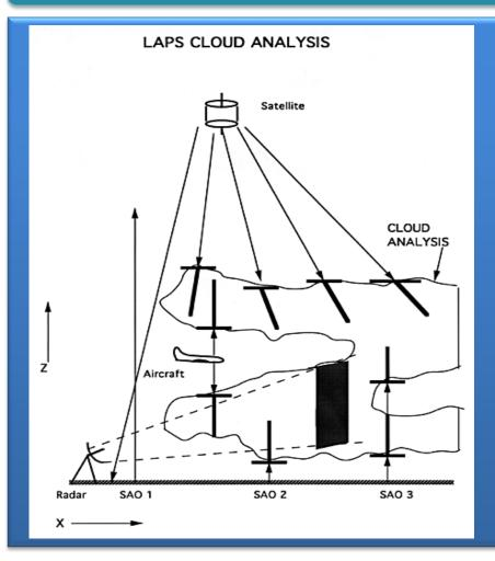
3D cloud distribution Cloud type 3D hydrometeor classification and surface precipitation Liquid and ice concentration
