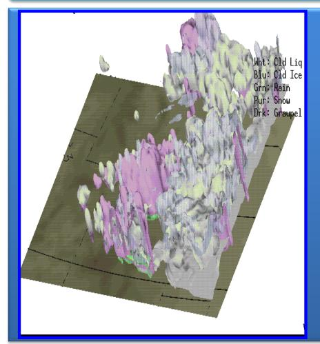
Dual-pol radar data play an important role in precipitation and cloud analysis LAPS system is upgraded to accept dual-pol radar parameters (ZDR, KDP and RHV) to better capture heavy rainfall and diagnose hydrometeors, especially hail events Additionally, many instability indices are calculated, which give the potential of the atmosphere to produce extreme weather events
